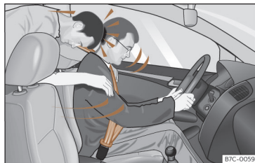
Fig. 41 Any rear seat occupants not wearing a seat belt may be thrown forward violently, hitting the driver who is wearing the seat belt.
