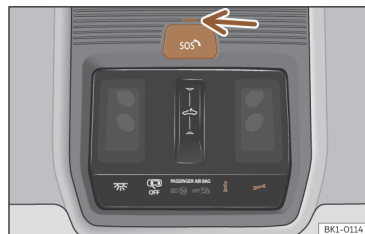
Fig. 64 On the roof console: controls for voice services.
