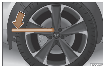
Fig. 200 Tyre change: slacken the wheel bolts.
