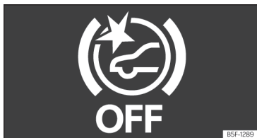
Fig. 135 On the screen of the instrument panel Front Assist switched off message.
