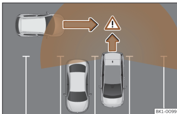
Fig. 144 Diagram of the parking assistant: detected area around the vehicle that is driving off.
