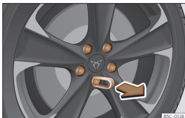
Fig. 198 Wheel: wheel bolts with caps.
